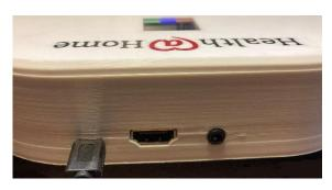
The PHG1500 is powered using the micro-USB connector (left). The PHG1500 also supports a display using the HDMI connector shown in this view (center). Audio is supported via the 3.5 mm jack (right).
