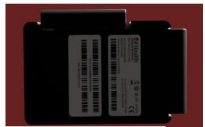
The label displays the serial number, model, and the sticker address used in configuring the hub (can also be scanned using the bar code) US FCC ID, Canada IC ID, CE mark, Japan Radio compliance
