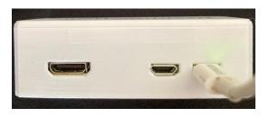
The PHG500 is powered using the micro USB connector (right). The PHG500 also supports a display using the HDMI connector shown in this view (left).
