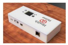
The PHG750 is powered using the micro USB connector (left). The PHG750 also provides an audio port for headphones and a mini-HDMI port
